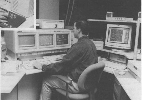
A SINGLE SAMPLE can be viewed by both Nancy Yang, above left, and technician Chris Rood, above, at the same time on separate workstations using the new digital microscopy system.
